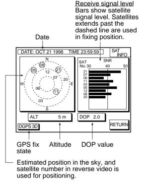
Figure 2-11 GPS satellite monitor display
